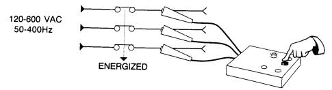
To identify the leads of a 3-phase motor, connect the tester to the de-energized motor, turn the motor in the desired direction, and press the test button. If the *reverse* LED glows, switch two leads and repeat. The *normal* LED should now glow. Label the motor leads according to the markings on the tester. NOTE the *loss* LED will glow during motor testing. This is normal since the turning motor generates less than 20 volts.
